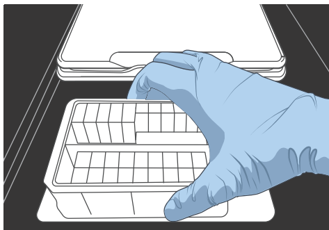
Figure 7 Placing Post Load Plate
